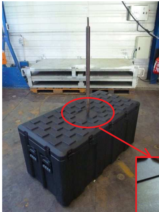
Photo 8: penetration test and marking of lid
